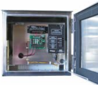
Compact cabinet holds time switch, solar regulator, flasher/fuse board and battery.
